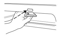
If the tether strap is clipped incorrectly (as shown) the child safety seat may not be retained properly in the event of a collision.
